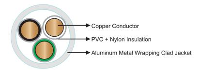
Conductor: Soft annealed bare copper, Class B stranding per ASTM B8
